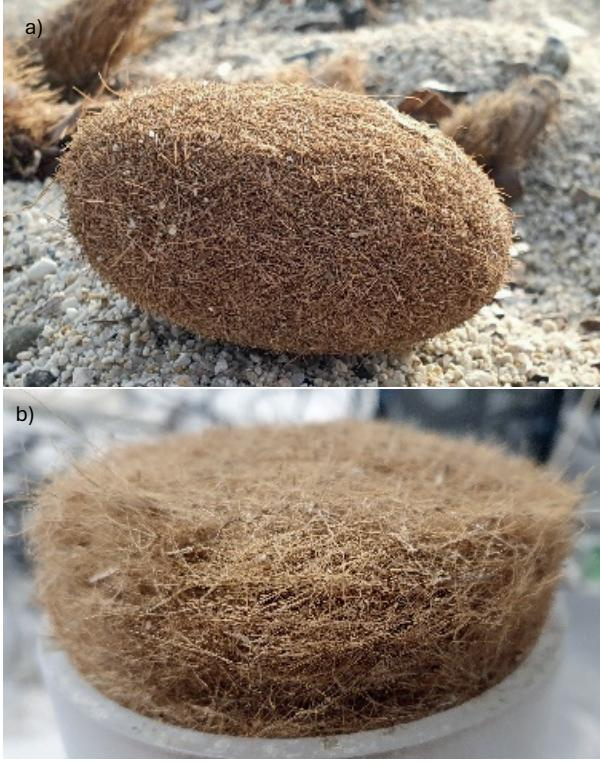
**Fig. 6 – Posidonia oceanica fibres: a) Aegagropiles deposited on the beach by the sea; b) Fibrous sample tested in the laboratory**
