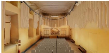
**Fig. 4 – Second designed solution with parametric baffles**
