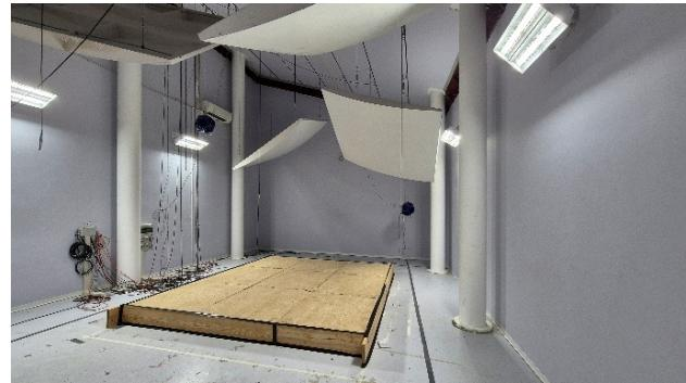
**Fig. 2 – Testing sample installed into the reverberant chamber**
