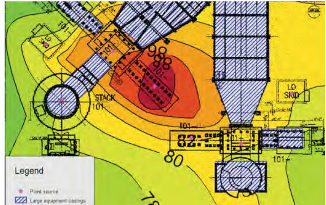
**Fig. 15 – Enlargement of the ammonia plant measured noise map on the induced and draft fans of “reformer” area**
