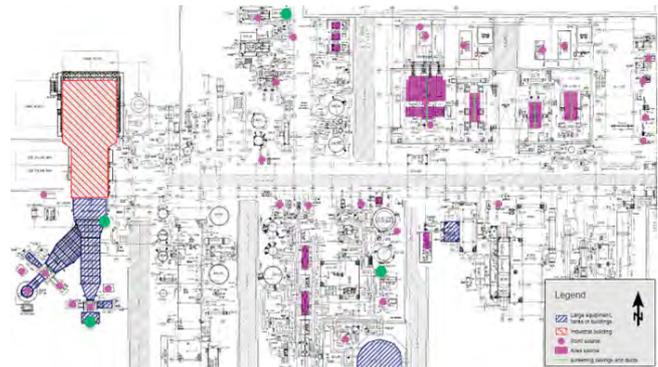
**Fig. 17 – Ammonia plant as built acoustic model: sources at design stage are fuchsia, 4 added sources are marked in green**
