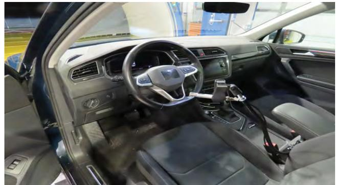
**Fig. 12 – Diffuse field microphone installation inside the car**
