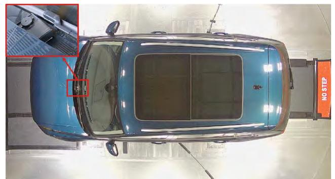
**Fig. 13 – KingState KPE-141 noise generator installation**
