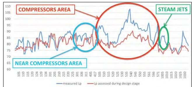
**Fig. 26 – Discrepancies between assessed and measured sound levels in dBA at measurement points, for numbering system see para. 2.4**
