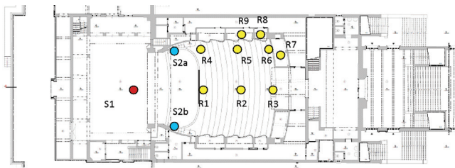
Fig. 7 – Source and measurement positions in the stalls (R1 – R6), in the central stage (R7) and in the lower side lodges (R8 and R9); S1 = position of the impulse source; S2a,b = positions of the two loudspeakers
