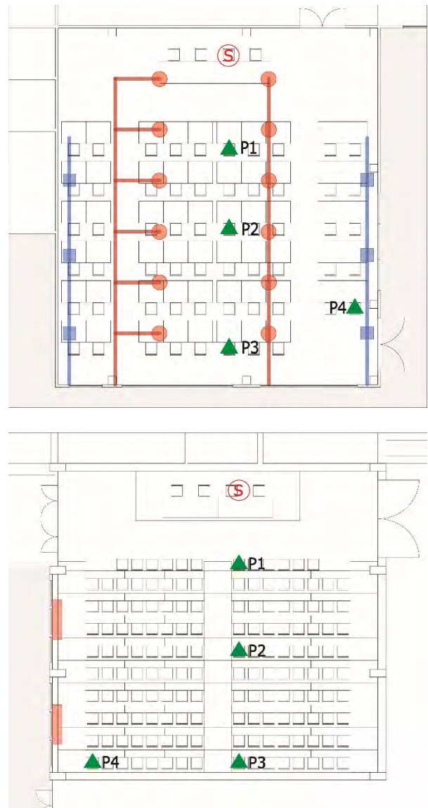
Fig. 4 – Posizioni microfoniche per la misura del C_{50} e del rumore impiantistico - Aula T2 (in alto) ed aula IE (in basso) Positions of the microphone for the measurement of C_{50} and noise from the thermal systems – Room T2 (top) and room IE (bottom)
