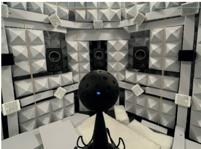
Fig. 12 – Setup di misura con Eigenmike® a 64 canali Measure setup with 64 channels Eigenmike®
