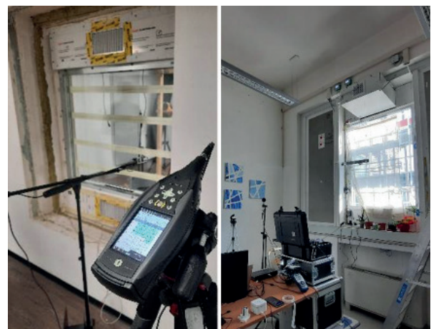
Fig. 2 – Laboratory and in situ test of sound reduction index R Misure in laboratorio e in situ del potere fonoisolante R
