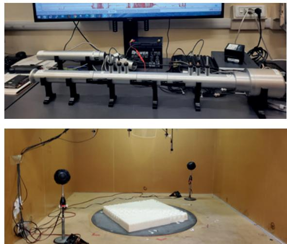
**Fig. 1 – Acoustic characterization: transmission loss in impedance tube (a) absorption in scaled reverberant chamber (b)**
