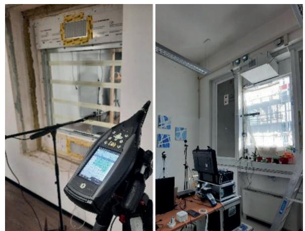
**Fig. 2 – Laboratory and in situ test of sound reduction index R**
