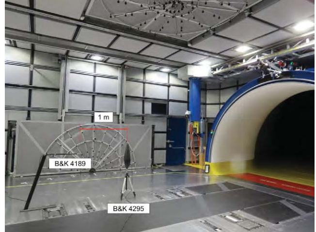
Fig. 5 – Side and overhead array validation test case experimental set-up
