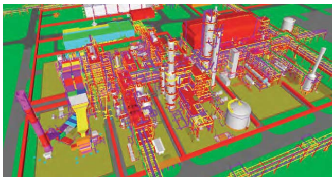
Fig. 1 – 3D model view of the ammonia plant. From left to right, there are the reformer package with its stack at the leftmost corner, the large pumps area in the middle and the compressor house behind the plant area on the right
