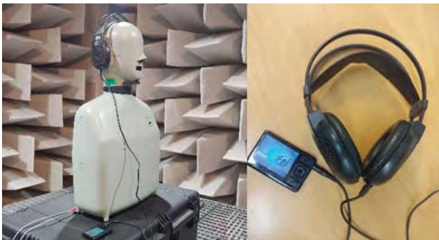
Fig. 1 – Calibration of the sound reproduction system used for the listening tests
