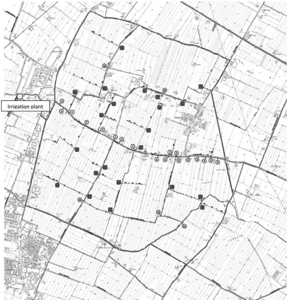
Figure 4 - Staggia Plant – irrigation pipe network
